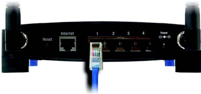
Figure 4-2: Connecting Your Network Devices
