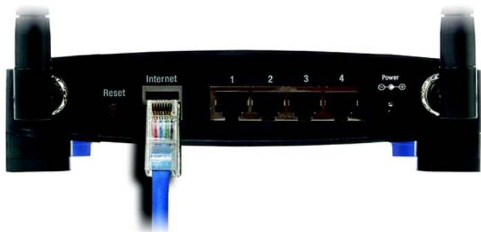
Figure 4-5: Connecting Another Router
